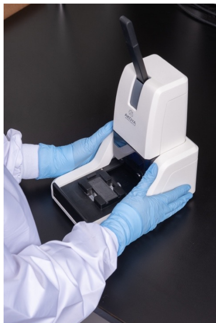
Figure 3.5. Correct handling of the assembly device using the lower shoulders.
