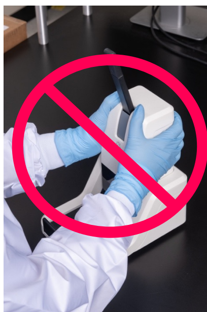
Figure 3.6. Incorrect handling of the assembly device using the central cover.
