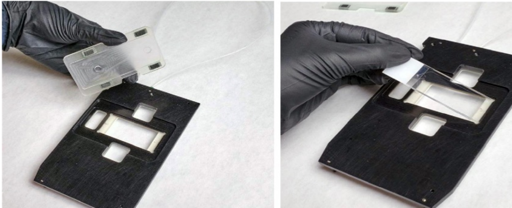
Figure 3.19. Carrier as the Magnetic Slide Retainer is being removed (left). Carrier being loaded with a Flow Cell Slide (right).
