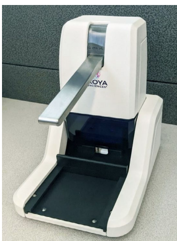
Figure 3.17. Assembly Device when the handle is completely pressed down.
