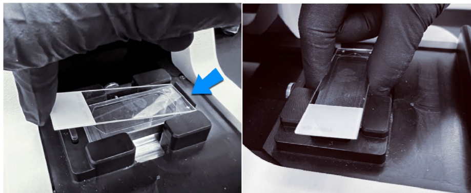
Figure 3.15. Placing the slide tissue-side down on top of Flow Cell with the non-label side against the stop bar, as indicated by the blue arrow (left). Aligning the slide and the Flow Cell (right).
