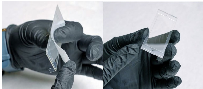
Figure 3.10. Remove the plastic cover slide (left) to reveal a Flow Cell without protective plastic cover (right).
