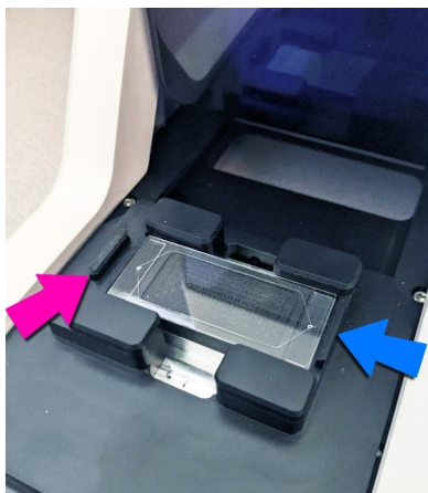
Figure 3.13. Flow Cell placed in the pocket of the Assembly Device with adhesive side facing up. The pink arrow on the left points to the spacer bar; the blue arrow on the right points to the stop bar.
