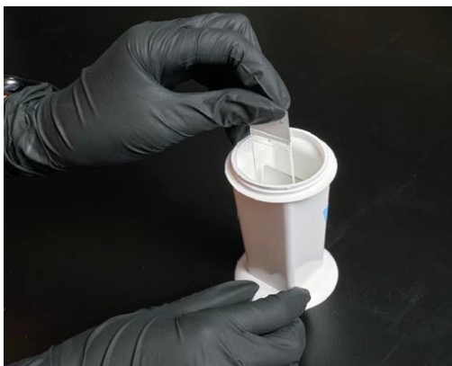
Figure 3.18. Adhered Flow Cell placed vertically in Coplin jar with 50 mL of 1X PhenoCycler-Fusion Buffer.
