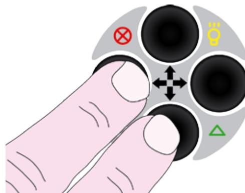
Use **Escape** to step out of a menu or to interrupt an ongoing Kermit communication. Press both buttons simultaneously according to the image.
