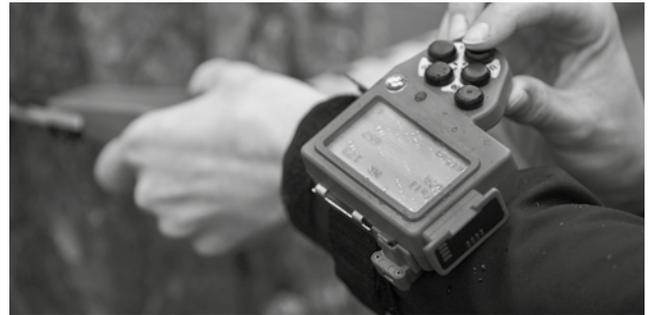
The DP II Computer Terminal can be detached from the moveable handle and the SmartScale. This is practical for example when transferring data to your office PC.
