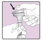
3) Hold the tube upright. Unscrew the funnel from the tube.
