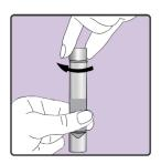
5) Shake the capped tube for 5 seconds. Discard the funnel.
