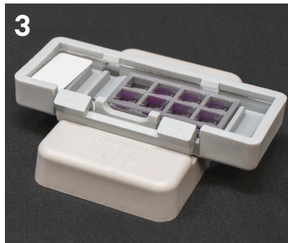
Visium Cassette sits securely on alignment tool
