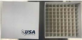
b. Create slots measuring 26 mm  $\times$  14 mm by removing every other insert in one direction.
