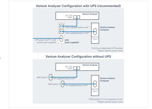
UPS should be plugged into an independent circuit. Refer to the user-acquired UPS installation documentation for UPS input circuit requirements.
