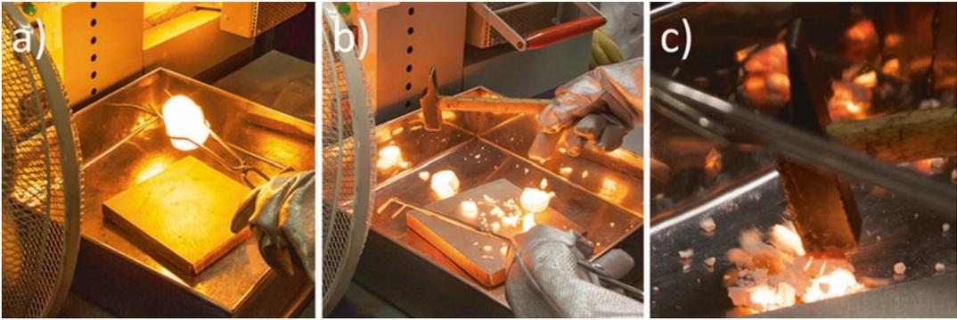
**Fig. 7** Steps followed for quenching of the  $\alpha$ -TCP. (a) Flip the crucible to extract the block, (b) the second person closes the furnace door and the operator breaks the block with a metallic hammer. (c) Detail of how the  $\alpha$ -TCP particles are broken with the hammer impact
