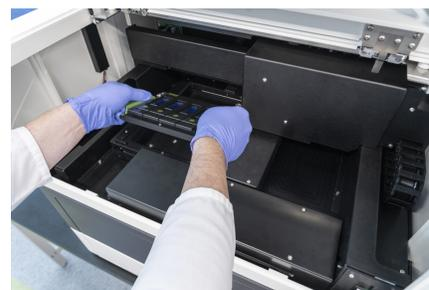
Figure 55: Unloading the slide holder
