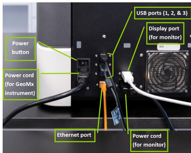
Figure 105: GeoMx DSP backside diagram
