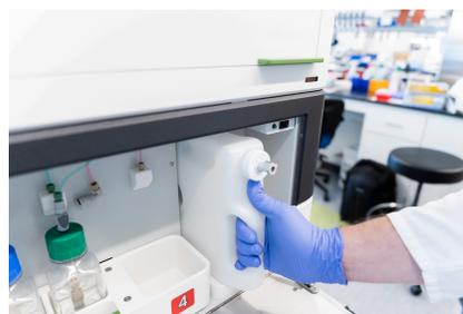
Figure 104: Removing GeoMx DSP waste
