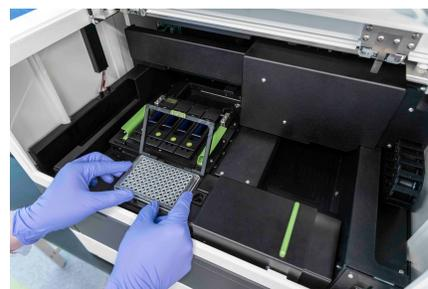
Figure 54: Unloading the collection plate on-on
