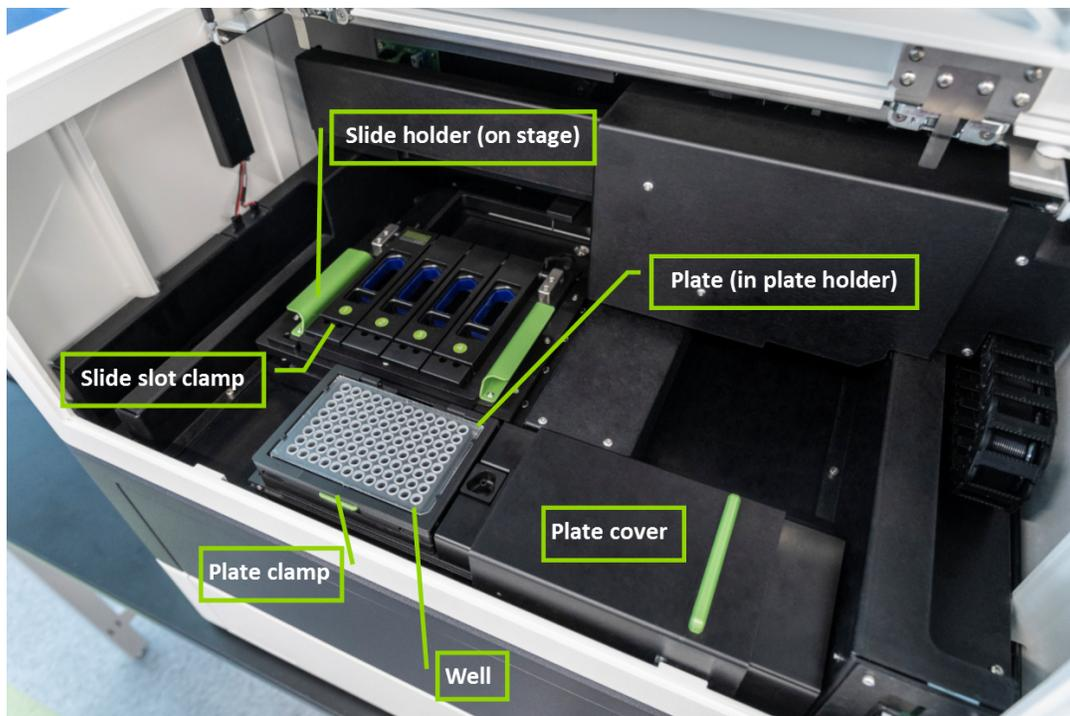
Figure 2: GeoMx DSP instrument interior diagram
