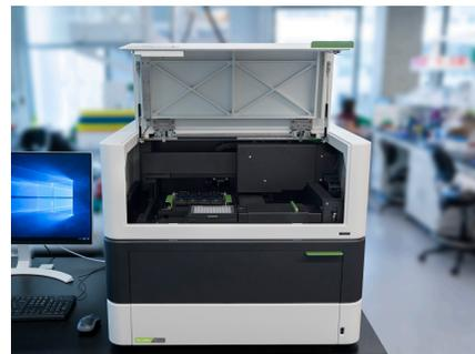
Figure 11: Open the GeoMx instrument door when prompted
