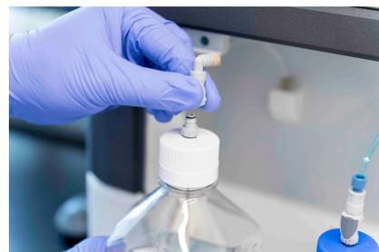
Figure 102: Disconnecting GeoMx reagent bottle
