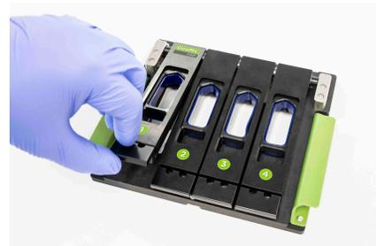
Figure 9: Lowering the slide holder clamps
