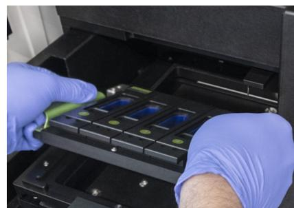
Figure 15: Insert the slide holder onto the stage of the instrument when prompted
