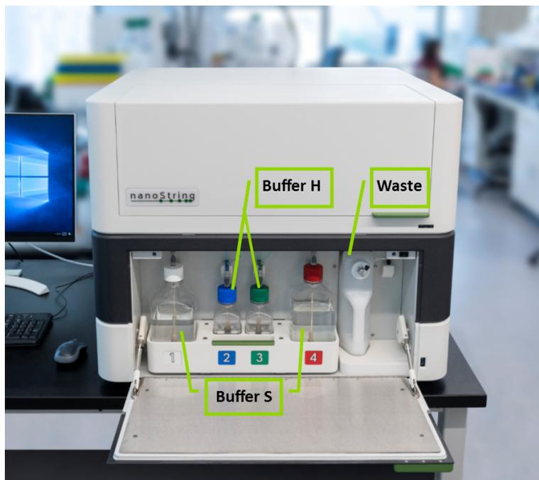
Figure 3: GeoMx DSP instrument reagent bay diagram
