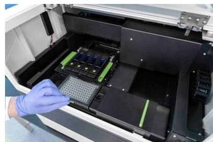
Figure 13: Fasten the clamp on the collection plate
