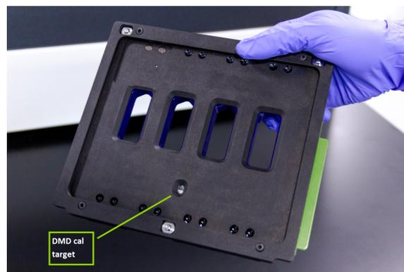
Figure 106: Underside of slide holder with DMD calibration (DMD cal) target indicated
