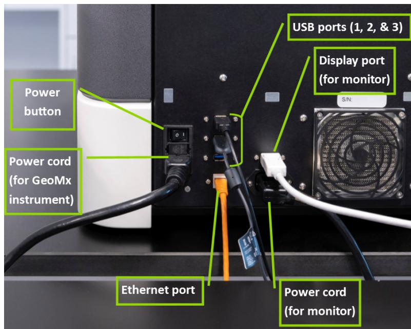
Figure 4: Diagram of back of GeoMx DSP instrument
