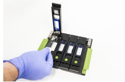
Figure 8: Loading the slide holder
