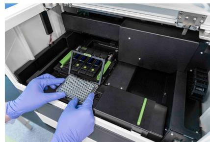
Figure 12: Insert the collection plate onto the plate holder when prompted
