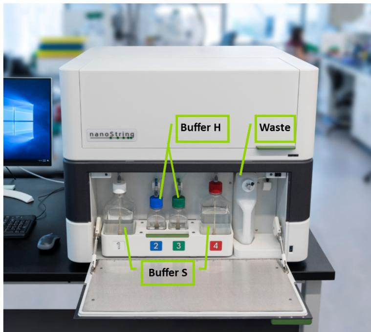
Figure 100: GeoMx DSP instrument reagent bay diagram
