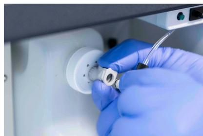
Figure 103: Disconnecting GeoMx DSP waste container
