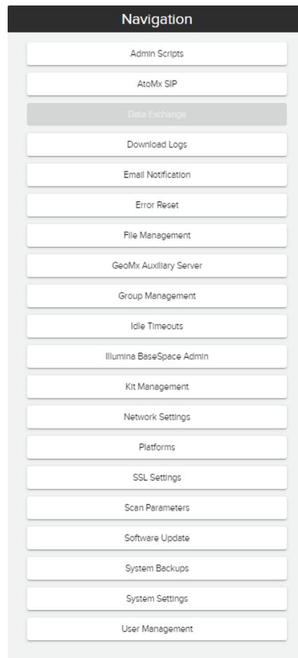
Figure 71 : GeoMx DSP Administration menu. Data Exchange is not available over remote connection.
