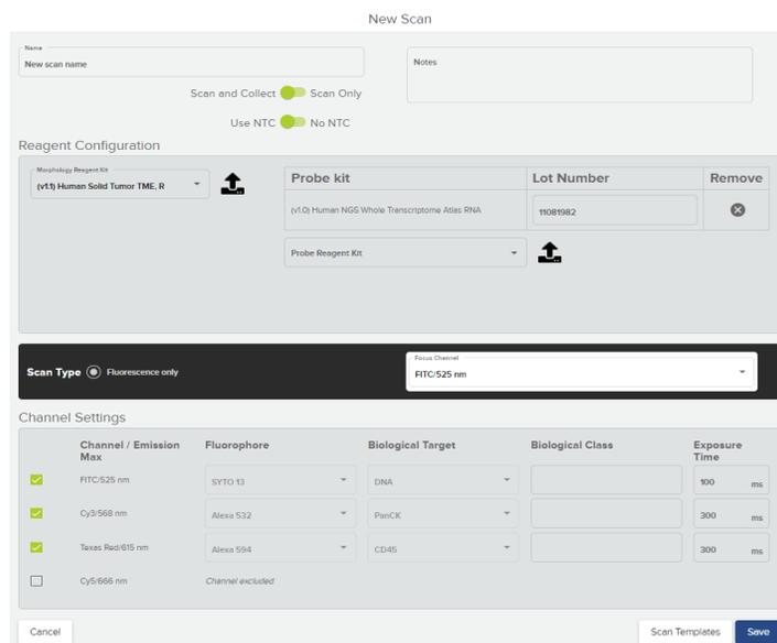
Figure 17: Scan parameters in Scan Configuration window
