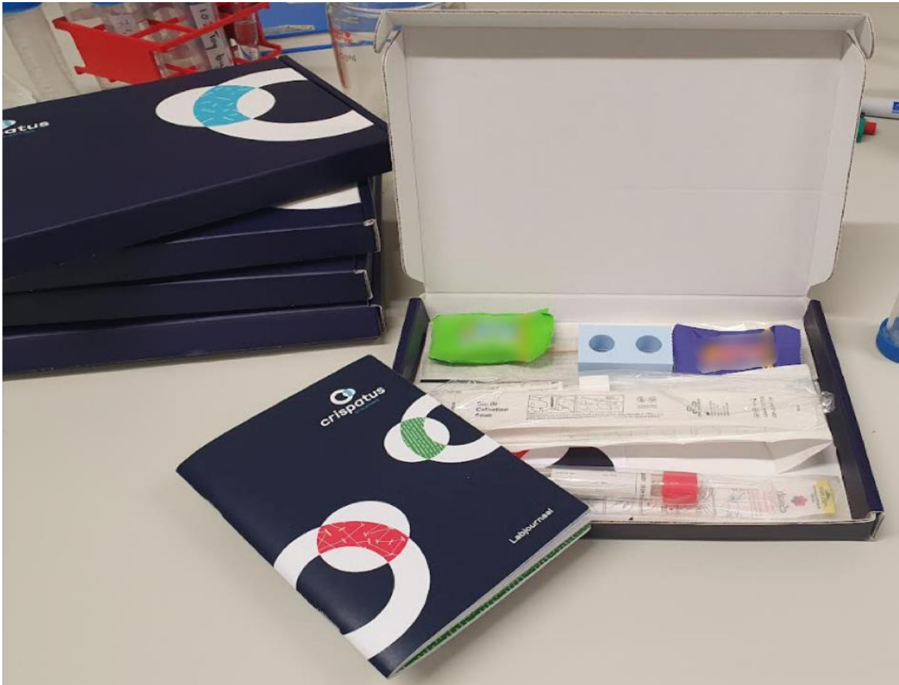
Figure 1 Content of a sampling kit, containing i) one collection tube with DNA/RNA shield buffer for metagenomic sampling; ii) one collection tube (e-swab) with Amies transport medium for isolation and microscopy; iii) a swab for a pH self-test; and iv) an information booklet that also served as a personal lab journal. Picture created by Rosanne Hertzberger, 2023.
