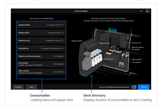
To aid in efficient and complete loading, the status of each item is shown on the left side of the screen and its location within the instrument deck is depicted on the right.
