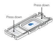
Apply even pressure on top of cassette until all clips click shut. Verify that clips are completely secured over tabs
