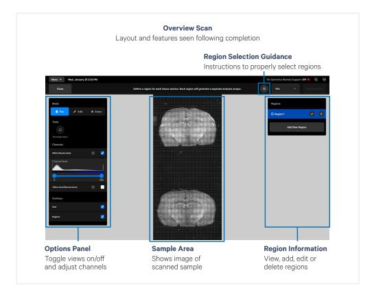
**c.** Review sample scan image. Use the panel on the left hand side of the screen to turn on/off channels, adjust channel levels, and view overlays.
