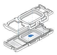
6 Add 1,000 µl PBS-T to cover the slide before loading onto the instrument
