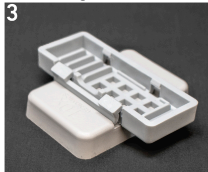
Visium Slide Cassette secured on alignment tool
