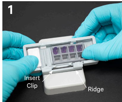
Position Visium Cassette along alignment tool ridges
