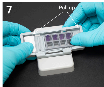
Remove Visium Cassette while pressing slide against the Visium Gasket
