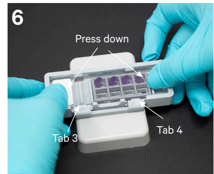
Press slide down until it is flush with the Visium Gasket and under tabs 3 & 4
