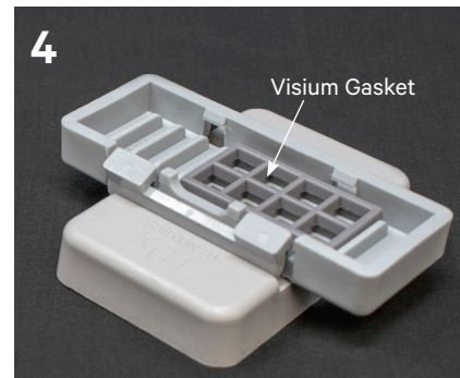
Position Visium Gasket to align with Visium Cassette cutouts
