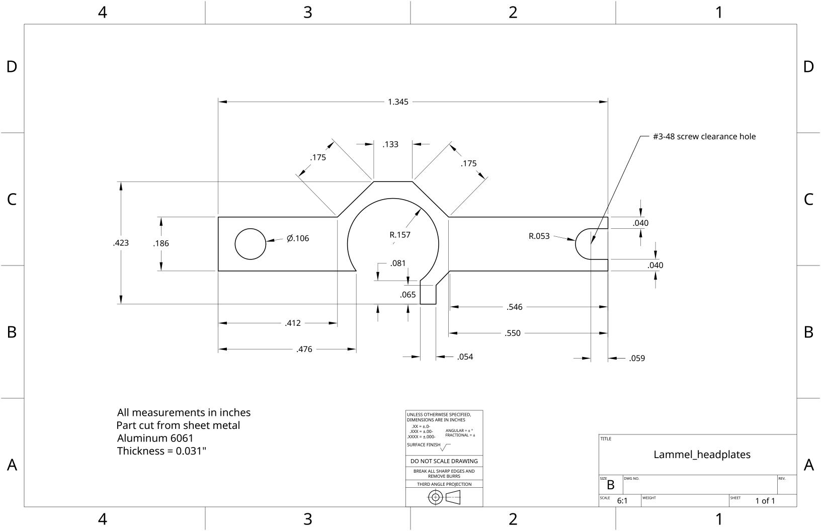
**Supplementary Figure 1. Specifications for headplate construction.** Details for lightweight headplates with clearance for neural implants on the surface of the skull and extended wings for head-fixation.
