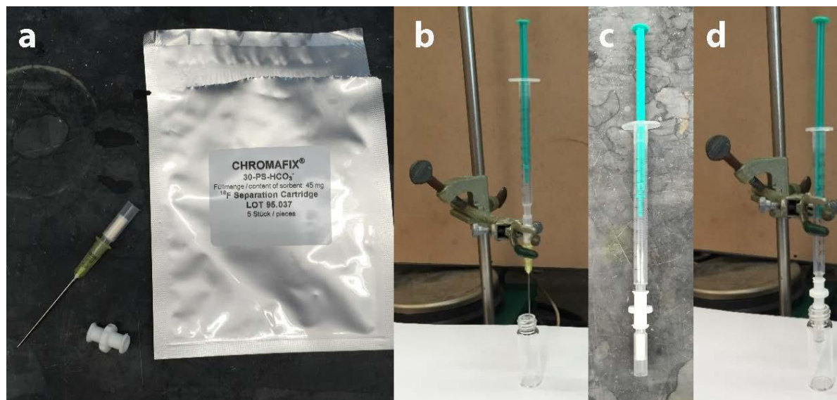
Fig. S10 | Photographs of the reverse elution workflow. a , A needle is affixed to a Chromafix cartridge; female-female luer adaptor b , Fluorine-18 loading set-up c , Cartridge fitted with a female-female luer adaptor d , Fluorine-18 elution set-up.
