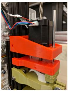
Received the non-captive steppers with Tr8-8 acme threaded rods, printed out new motor mounts out of PETG, should be better suited for the job as the motor heats up. Made sure that the threaded rod is supported within the mount. Kept 5mm guide rods, could potentially go for 8mm.
