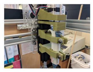
Unfortunately the 5 mm linear bearings that support the 5 mm rods may be inferior to the bronze bushings in the Opentrons robot. The linear bearings fit the rod tightly, however a moderate amount of force is enough to allow the rods to bend out
