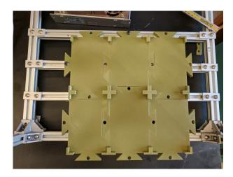
Here it is loaded up with different containers, I 3D printed the 4×5 1.5 mL tube holders in two parts and finally made some nice wedges to keep odd shape stuff snugly in each slot. Pretty reasonable amount of working room I think, we will see if I run into any trouble on that front.
