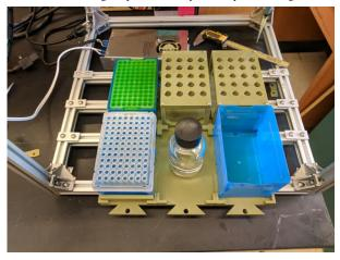
I've had a bit of issue with certain pipette tips being difficult to eject, I solved this issue by beefing up the pipette and motor mounts on the A axis. As well, I increased the length of the wedge that actuates the pipette eject.
