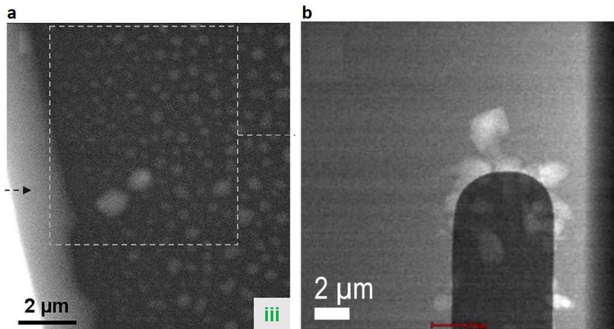
**Supplementary Figure 1 | Comparison of spatial resolution.** **a** | TEM image observed using electrochemical liquid cell of Hummingbird company. **b** | TEM image observed using electrochemical liquid cell of Protochips company. Part **a** is adapted with permission from ref.<sup>1</sup>. American Chemistry Society. Part **b** is adapted with permission from ref.<sup>2</sup>. Springer Nature Limited.
