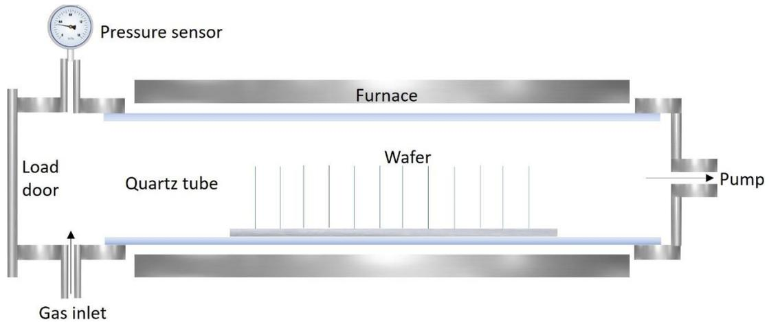
**Supplementary Figure 2 | Schematic illustration of the low-pressure chemical vapor deposition (LPCVD) setup.** LPCVD furnace. For the detailed information, the reader is referred to the Chapter 5.17 of the following link: ([https://nanolab.berkeley.edu/public/manuals/equipment\\_manual.shtml](https://nanolab.berkeley.edu/public/manuals/equipment_manual.shtml)).
