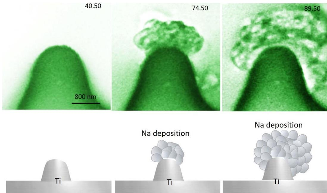
**Supplementary Figure 7 | In-situ TEM observation of Na electrodeposition on undulant Ti surface using electrochemical liquid cell III (Ti electrode, commercial NaPF<sub>6</sub>/PC electrolyte).** Top: sequential TEM images from **Supplementary Video 8**. Bottom: schematic illustration of Na electrodeposition on undulant Ti surface. The TEM images are adapted with permission from ref.<sup>4</sup>. Elsevier.
