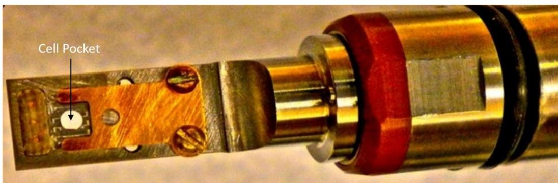
**Supplementary Figure 5 | Photo of the custom TEM holder.** The custom TEM holder provides a platform for fixing liquid cell and connecting the TEM equipment. There is a cell pocket at the TEM holder tip for placing liquid cell. Adapted with permission from ref.<sup>3</sup>. Royal Society of Chemistry.
