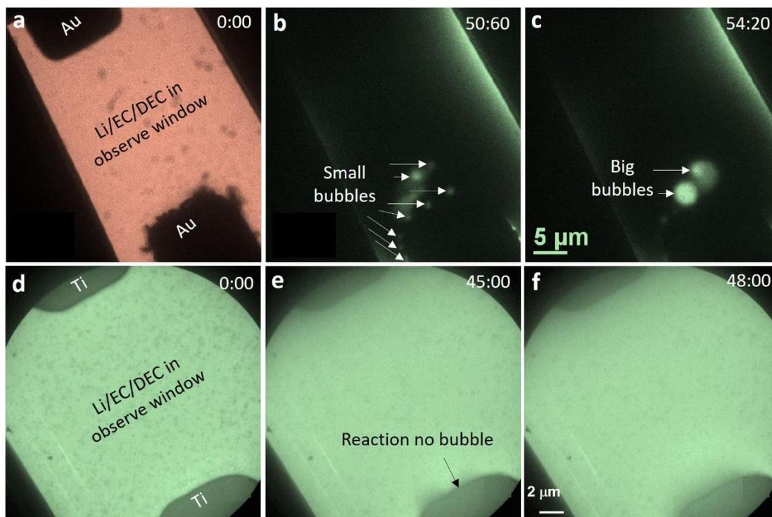
**Supplementary Figure 8 | Sequential images show the electrode-electrolyte interface reaction on both sides of the electrodes in two electrochemical cells. a-c | Au electrodes. d-f | Ti electrodes. Note that Au electrode has bubbles and the Ti doesn't. Adapted with permission from ref.<sup>3</sup>. Royal Society of Chemistry.**
