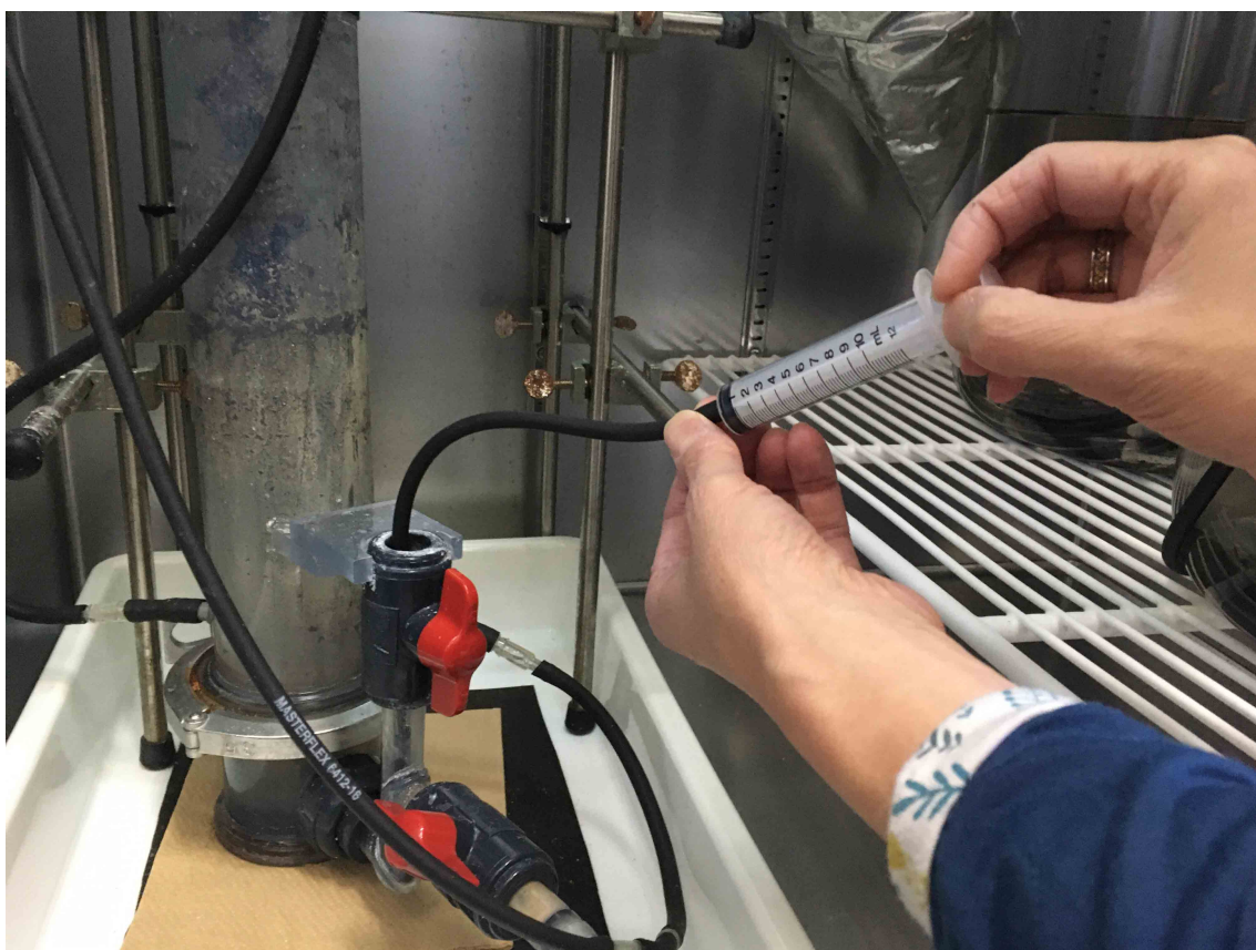
Supplementary Fig. 5| Effluent sampling using a 10-ml syringe attached with Viton tubing from the effluent pool in the bottom of the reactor column.
