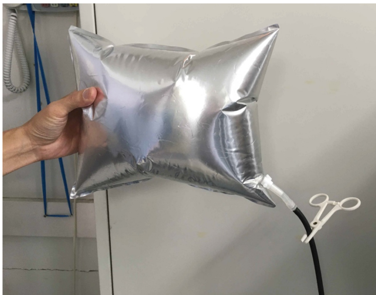
Supplementary Fig. 3| Aluminum bag and clamp. The image shows that a clamp is attached to the flow path between the influent gas bag and the reactor column.
