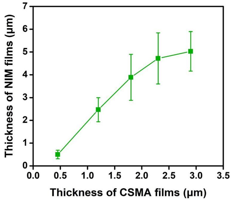
**Supplementary Fig. 3 The thickness relationship between the NIM film and the CSMA film.** As the thickness of the CSMA film increases, the thickness of the mineralized film also increases.
