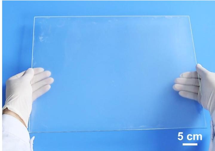
**Supplementary Fig. 1** Photograph of NIM film with a large-sized area of 30 cm × 40 cm.
