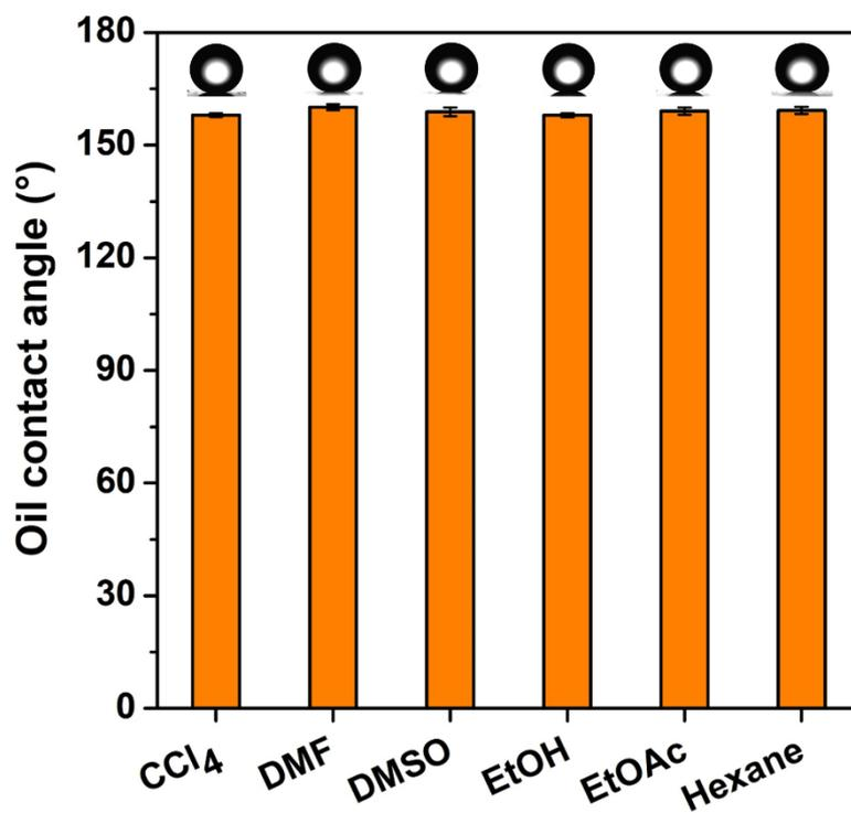
**Supplementary Fig. 2 Study of solvent resistance ability of the NIM film.** The underwater oil contact angles of the NIM film after immersing in various organic solvents for 24 h, including carbon tetrachloride (CCl<sub>4</sub>), dimethylformamide (DMF), dimethyl sulfoxide (DMSO), ethyl alcohol (EtOH), ethyl acetate (EtOAc) and hexane.
