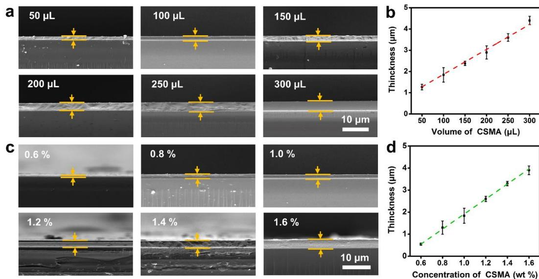
**Supplementary Fig. 5 The regulation of thickness of CSMA films.** a, c) SEM images of CSMA films with different thicknesses by regulating the volume and concentration of CSMA solution. b, d) The corresponding variation of film thickness with the volume or concentration of CSMA solution, which was fitting first order linear relation. **a-d** adapted with permission from ref.<sup>1</sup>, Wiley.
