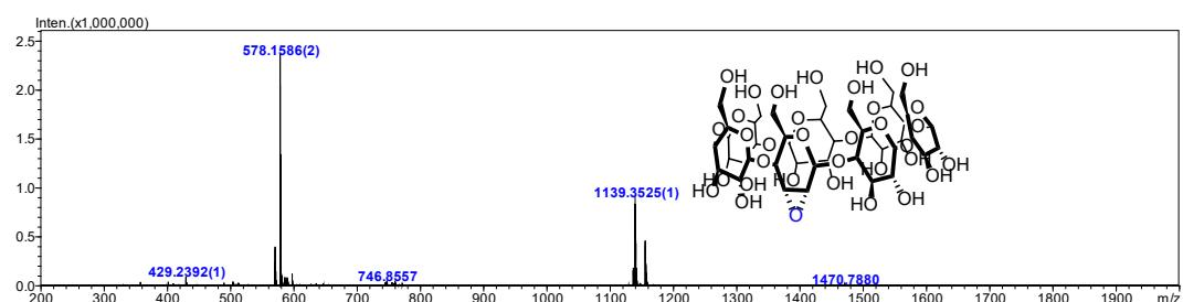
**Supplementary Figure 27.** HR-MS (ESI) spectrum of  $2^{\text{A}},3^{\text{A}}$ -alloepoxy- $\beta$ -CD 16.
