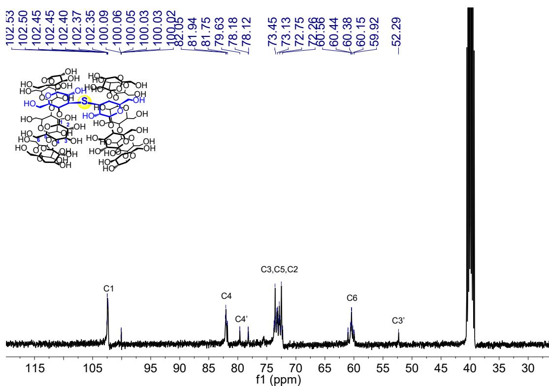
**Supplementary Figure 32.**  $^{13}\text{C}$  NMR spectrum of **10** (101 MHz,  $\text{DMSO}-d_6$ , 298 K).
