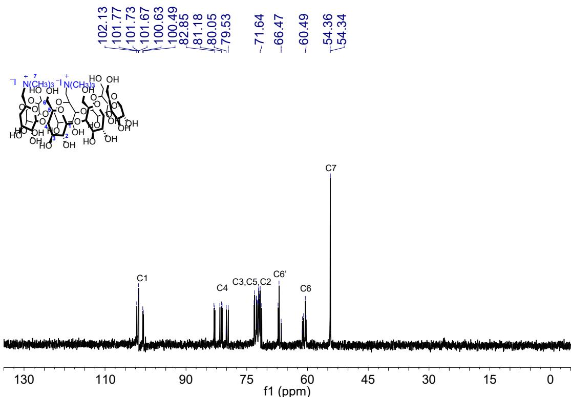
**Supplementary Figure 17.**  $^{13}\text{C}$  NMR spectrum of  $6^{\text{A}},6^{\text{C}}$ -TMA<sub>2</sub>- $\beta$ -CD **7** (101 MHz, D<sub>2</sub>O, 298 K).
