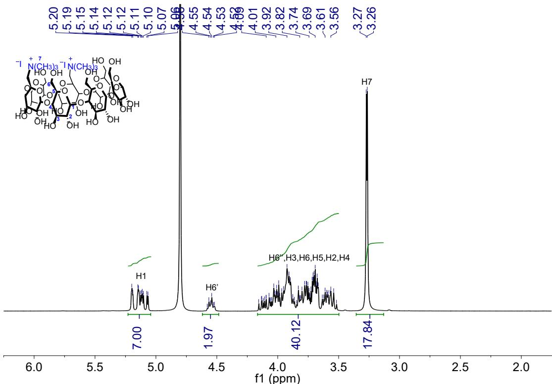
**Supplementary Figure 16.**  $^1\text{H}$  NMR spectrum of  $6^{\text{A}},6^{\text{C}}$ -TMA<sub>2</sub>- $\beta$ -CD **7** (400 MHz, D<sub>2</sub>O, 298 K).
