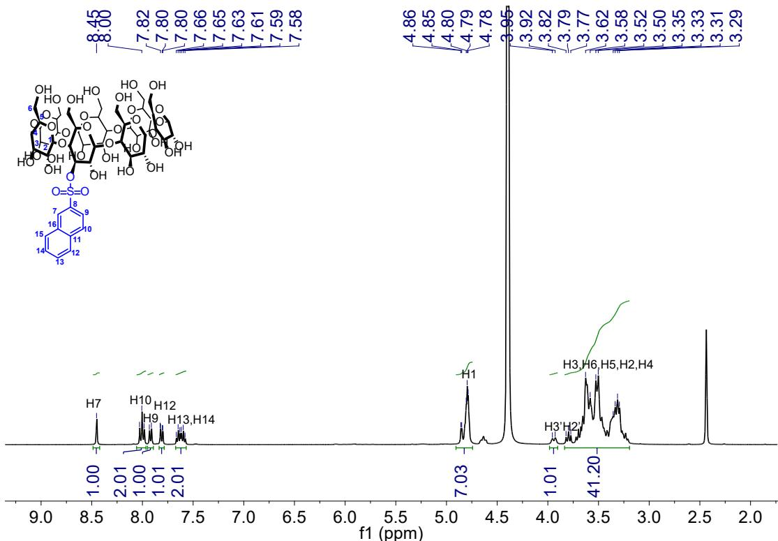
**Supplementary Figure 22.**  $^1\text{H}$  NMR spectrum of NS- $\beta$ -CD **15** (400 MHz,  $\text{DMSO}-d_6$ :  $\text{D}_2\text{O}$  = 1:1, v/v, 298 K).
