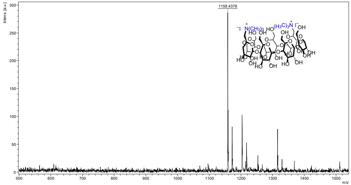
**Supplementary Figure 21.** MALDI-TOF mass spectrum of 6<sup>A</sup>,6<sup>D</sup>-TMA<sub>2</sub>- $\beta$ -CD **8**.
