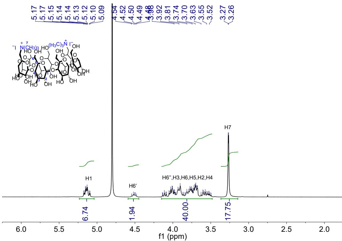
**Supplementary Figure 19.**  $^1\text{H}$  NMR spectrum of  $6^{\text{A}},6^{\text{D}}\text{-TMA}_2\text{-}\beta\text{-CD}$  **8** (400 MHz,  $\text{D}_2\text{O}$ , 298 K).
