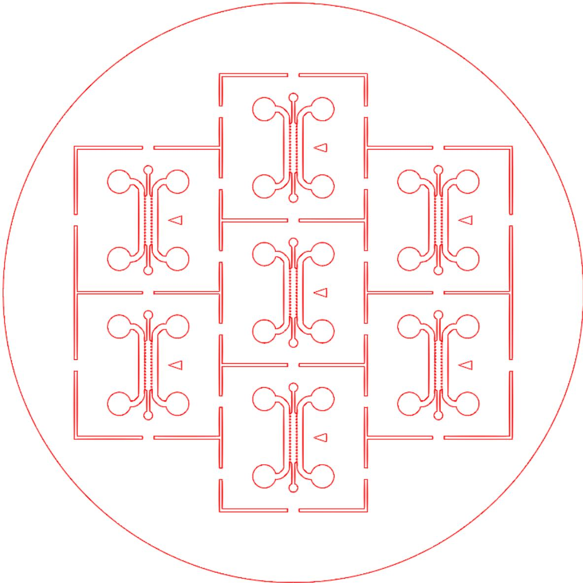
**Supplementary Figure 2.** Image of the CAD template for the micro device. CAD file is included in Supplementary Data 2.
