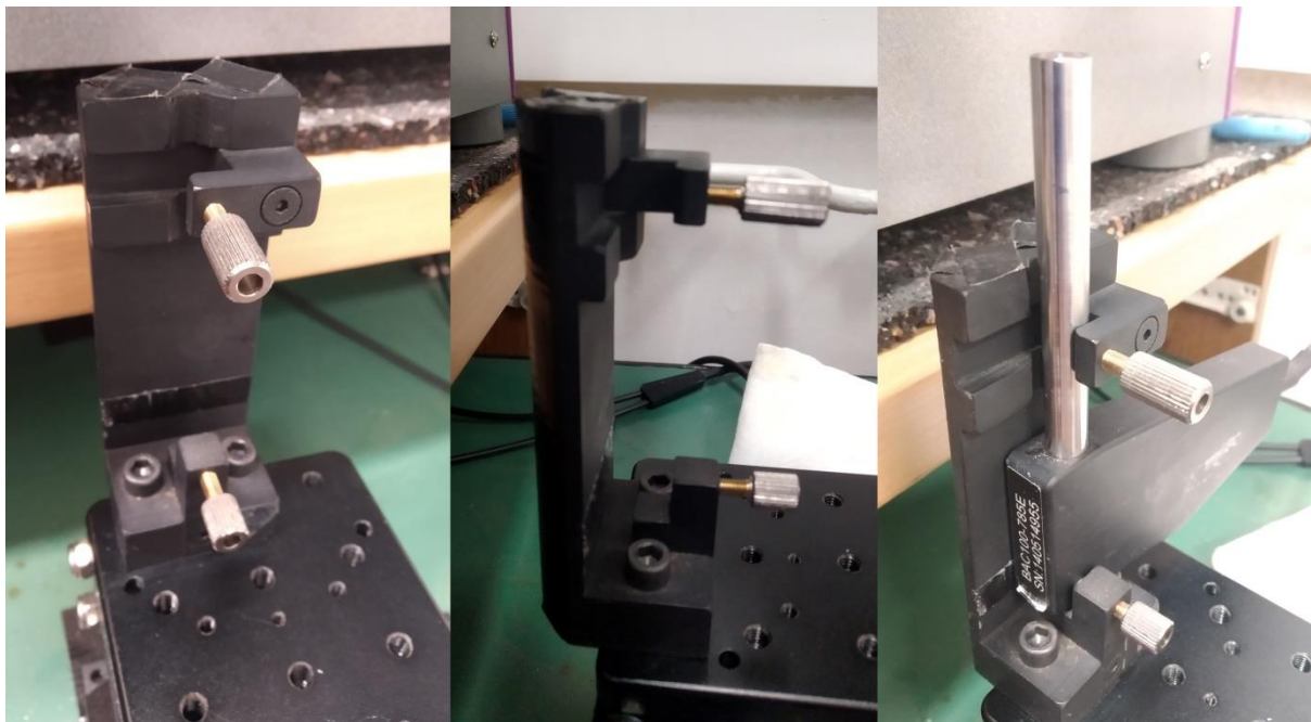
Supplementary Figure 3. Close-up of Raman probe holder without and with the mounted probe.
