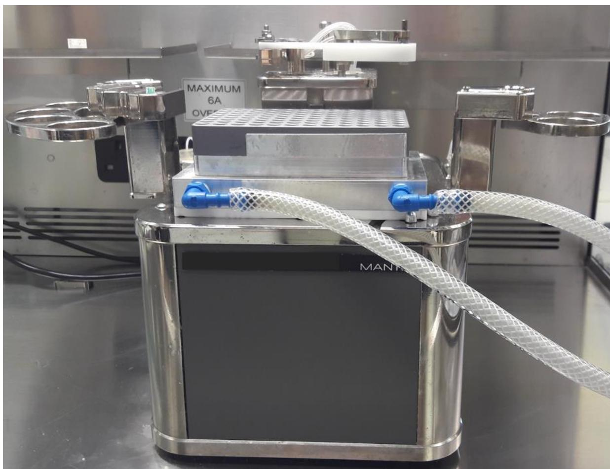
Supplementary Figure 2. Formulatrix Mantis microfluidic liquid handler
