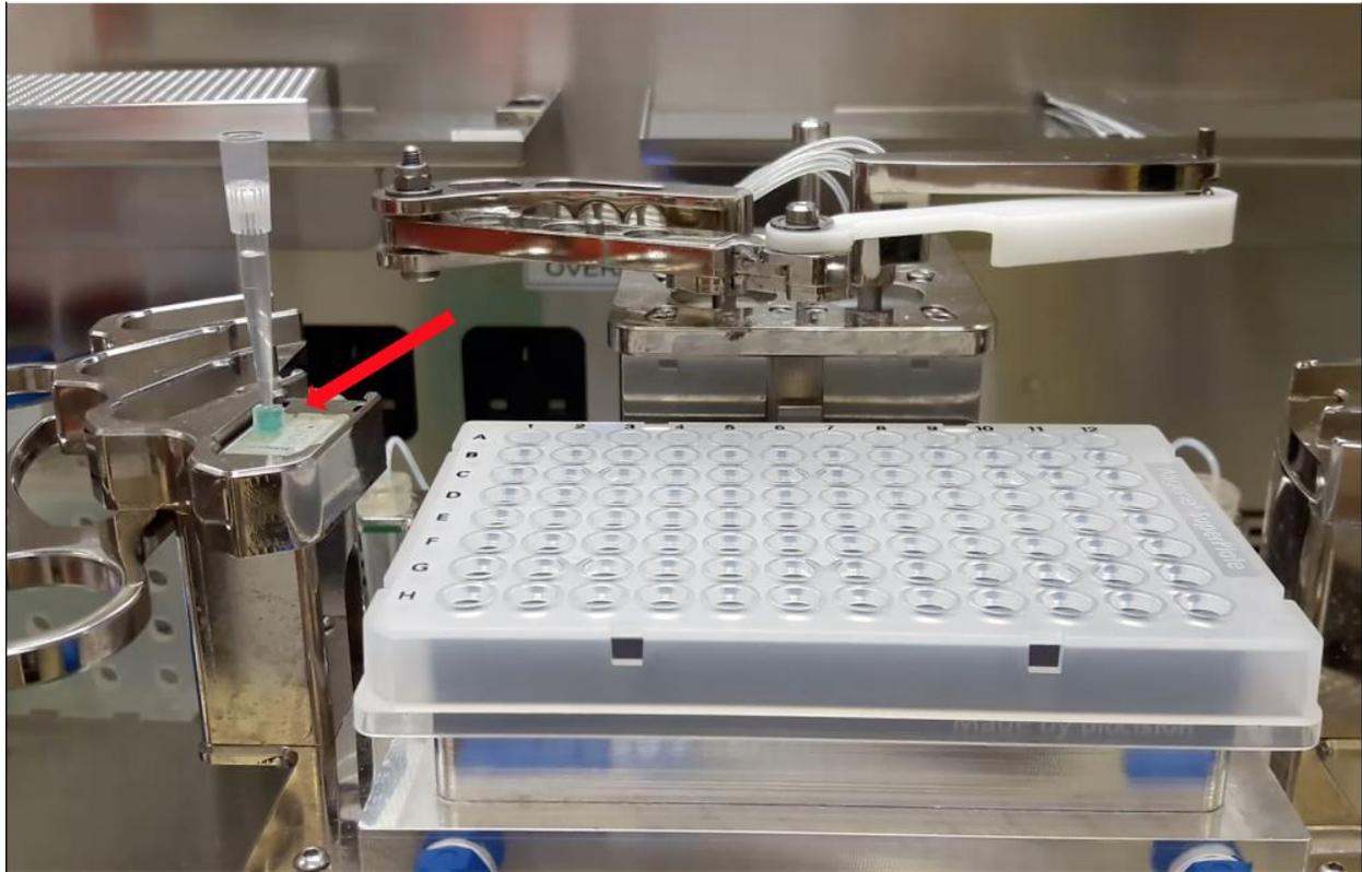
Supplementary Figure 4. Reagent dispensing on the Formulatrix Mantis microfluidic liquid handler.
